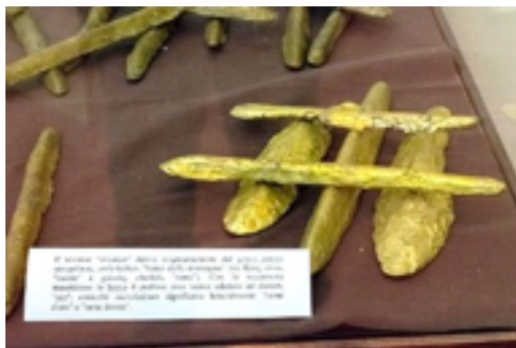
Ingots found in a shipwreck near Gela, Sicily, in the Gela Museum, labeled as orichalcum. They are an alloy of copper, zinc, nickel, lead, and other metals. Photo by Emanuele iela, via Wikimedia Commons.
