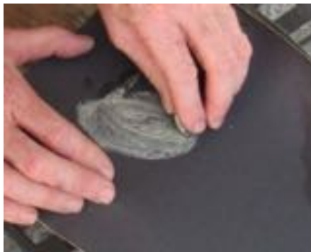
Smoothing and polishing a piece of amber with 220-grit sandpaper.
